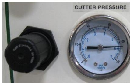
**Cutter pressure regulator** Will increase and decrease the pressure of the cutter. To increase the pressure turn the knob clock wise and to decrease the pressure turn the knob counter clock wise. When decreasing the pressure it is recommended to turn the pressure to zero then increase to the correct pressure.
