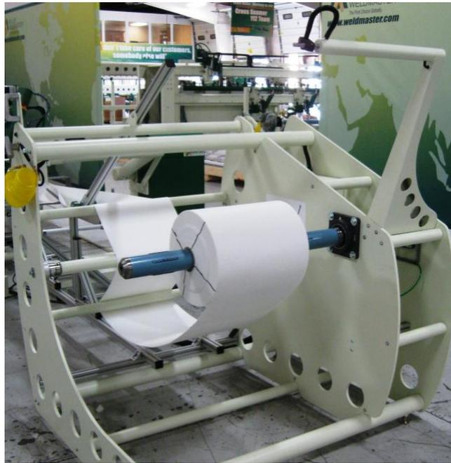
**Unwind stand** The unwind stand will hold the roll of material. The machine runs off of tension. The unwind stand will keep the tension while the machine is running. The tension is controlled by the tension roller connected to the load cells.
