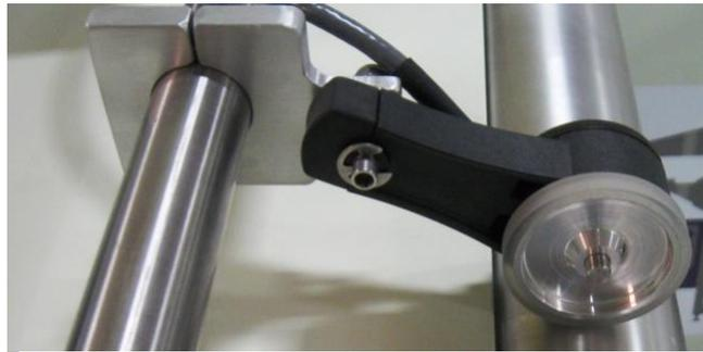
**Encoder** The encoder will only be used for lengths shorter than 2 feet and lengths longer than 15 feet. The settings for the encoder will be found on the machines HMI.
