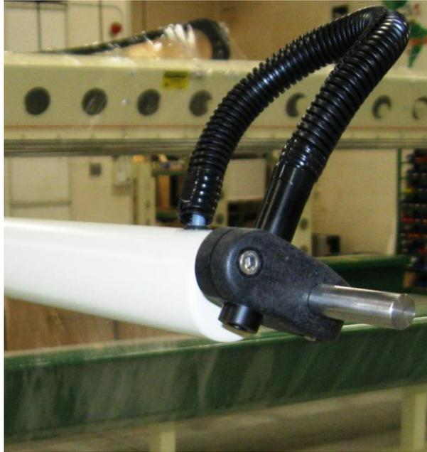
**The laser line.** The laser line will allow the operator to quickly line up new rolls. The laser line is the center line of the machine that all measurements are made from.
