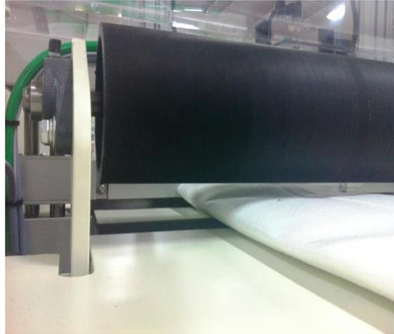
**Conveyor puller roller** The puller roller will pull from the accumulator. The speed of the puller roller is determined by the position of the accumulator. The open/ close button is located on the HMI screen.
