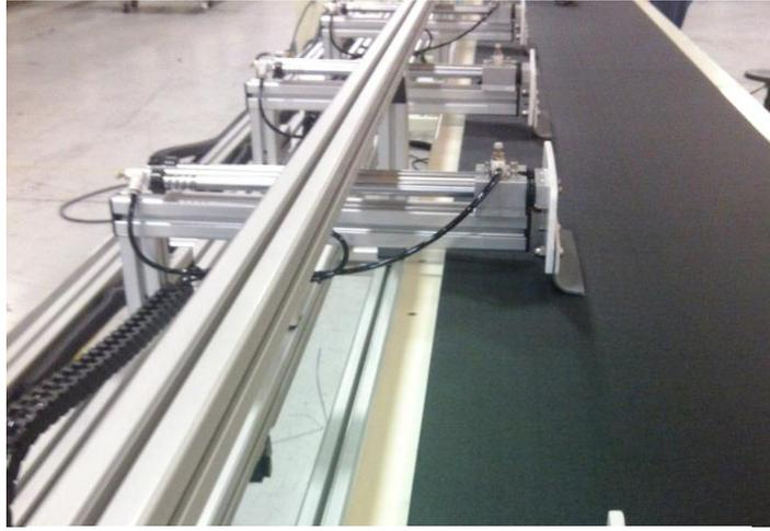
**Sweeping system** The sweeping system will push the material off the conveyer. The sweeping system is controlled by the cut. After the cut there is an adjustable timer that will trigger the sweeping systems. Each sweep can move left to right to accommodate and length of material. Each sweep can individually be turned on and off.
