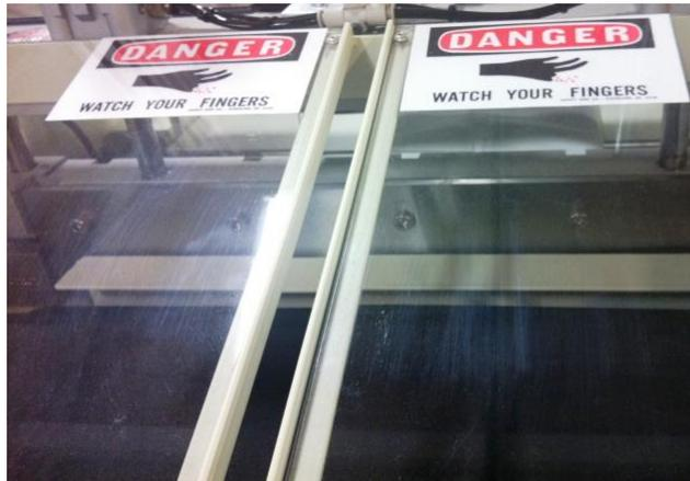
**Guillotine Cutter** will cut the material at desired length triggered by the Cut to Length Photo Eye Sensor.
