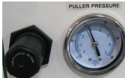
**Puller pressue regulator** Will increase and decrease the pressure of the puller. To increase the pressure turn the knob clock wise and to decrease the pressure turn the knob counter clock wise. When decreasing the pressure it is recommended to turn the pressure to zero then increase to the correct pressure.
