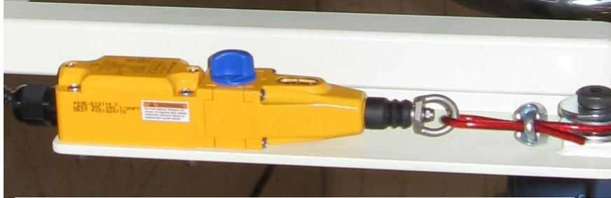
**Rope pull e stop** Will shut off power to any moving part of the machine. Once the rope pull has been pulled you must reset by turning the blue button back to the forward arrow.
