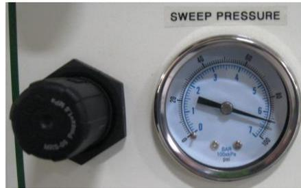
**Sweep pressure regulator** Will increase and decrease the pressure of the sweep system. To increase the pressure turn the knob clock wise and to decrease the pressure turn the knob counter clock wise. When decreasing the pressure it is recommended to turn the pressure to zero then increase to the correct .pressure.
