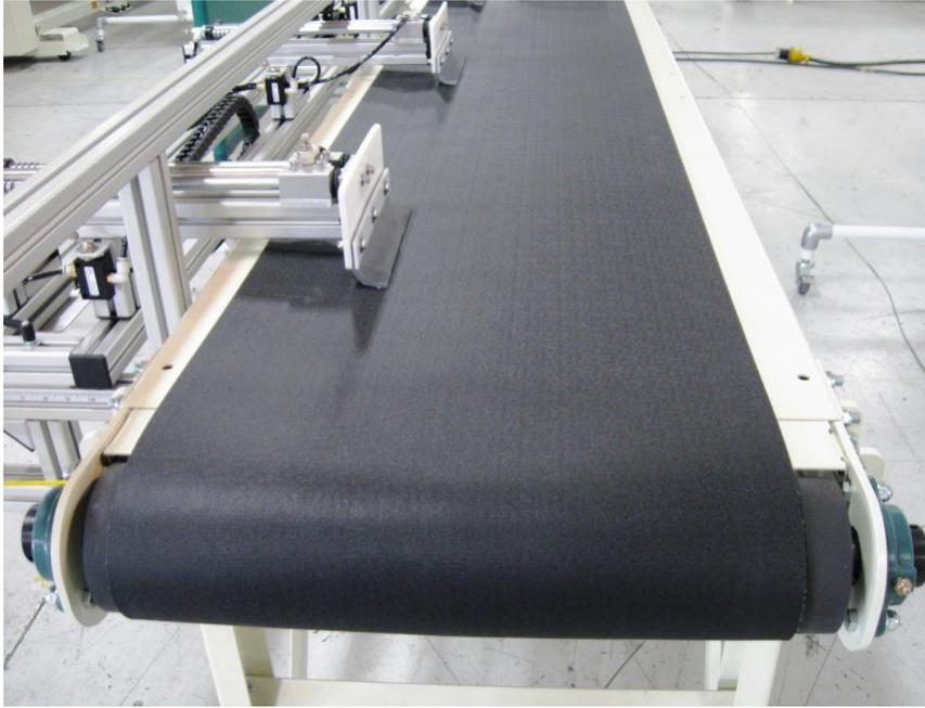
**Conveyer** Will Move the Material To cut length. And feed out the end for finished product.
