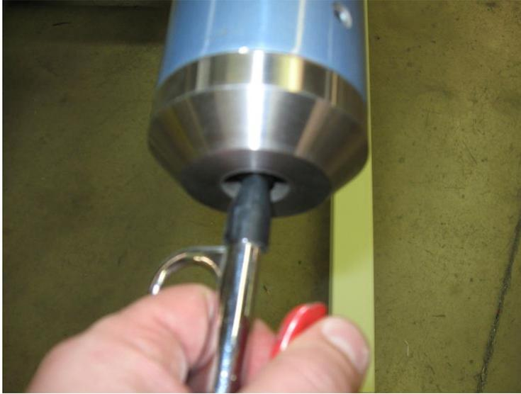
**Airing the shaft** The shaft must have air in it to hold the roll of material in place. The above picture shows where you air the shaft and release the air. Place the air nozzle in the shafts air valve to inflate. To deflate the air shaft hold in the valve till all the air is released.
