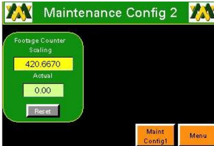
**Footage counter scaling** Will increase or decrease the length of the material. It is recommended to contact Miller Weldmaster before making any adjustments to the scaling factor.
