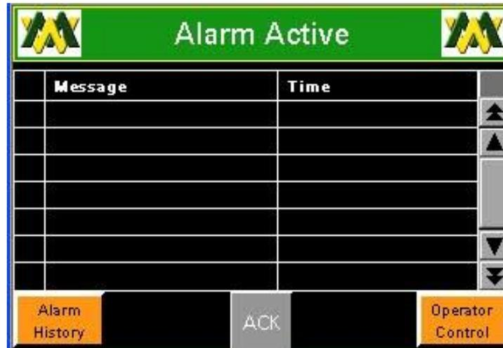
**Alarm Screen.** Displays any alarm that may have occurred. The button tells the machine that you recognized the problem and the proper adjustments have been made. You must push the ack. button to continue to run.
