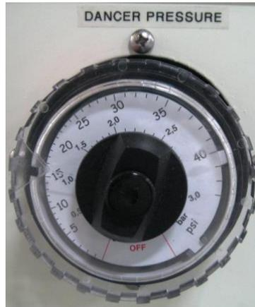
**Dancer pressure regulator** Will increase and decrease the pressure of the sweep system. To increase the pressure turn the knob clock wise and to decrease the pressure turn the knob counter clock wise. When decreasing the pressure it is recommended to turn the pressure to zero then increase to the correct.
