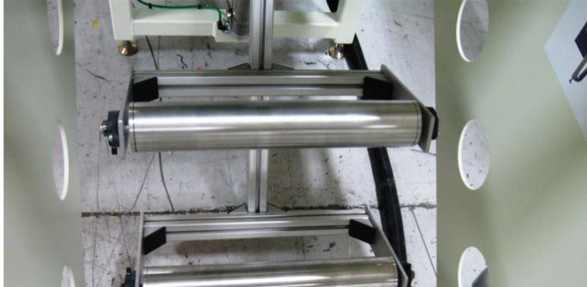
**Accumulator** The accumulator is used for a continuous process. As the material is being cut, the accumulator will take up any slack while the machine is being cut so that the machine doesn't stop the welding process.
