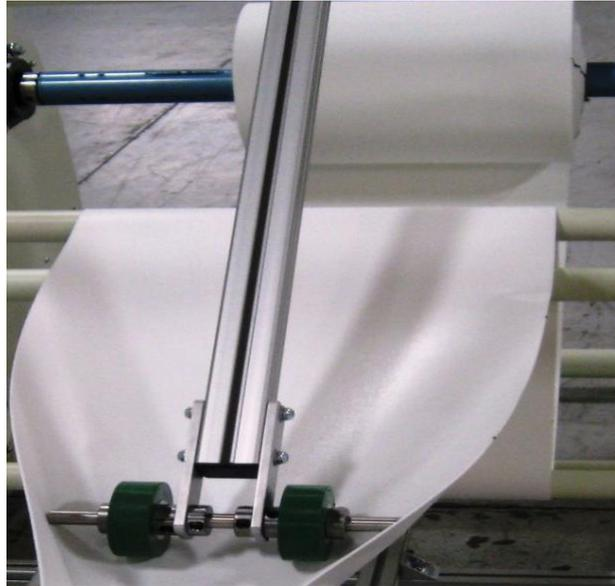
**Drop Roller** The drop roller will start the folding process of the tube. The drop roller is adjustable for different widths. The drop roller will adjust for the tubes lay flat
